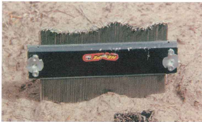
Figure 5. A. Rugosity-measuring device on a surface that appeared devoid of cryptogams on the managed area at Largo Mesa. B. The trace used to measure variation in the ground surface (see text).
