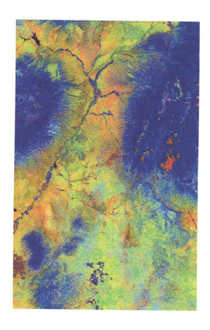
Figure 5. Band ratio image. FEOI in red, RI in green, and CI in blue.
