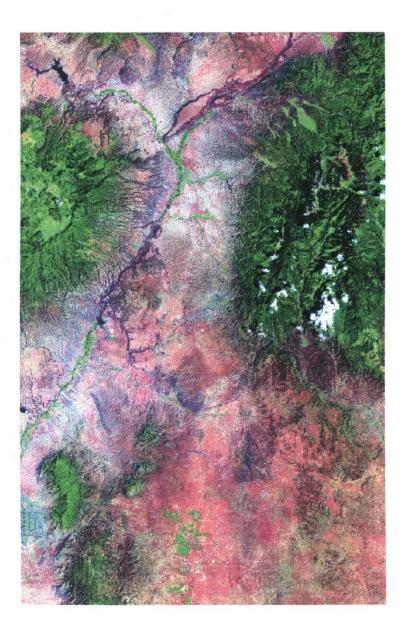
Figure 3. Landsat TM bands 5,4, and 2 shown in red, green, and blue.
