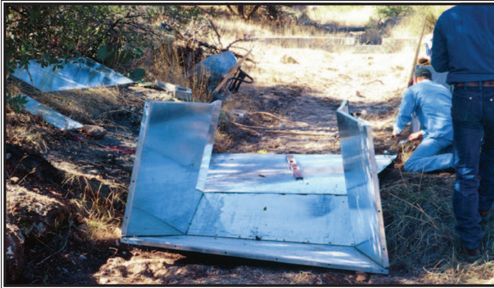
Prefabricated steel flumes, which can be assembled in the field, have been used to measure streamflow in remote, relatively inaccessible areas. (Photo by Gerald Gottfried)
