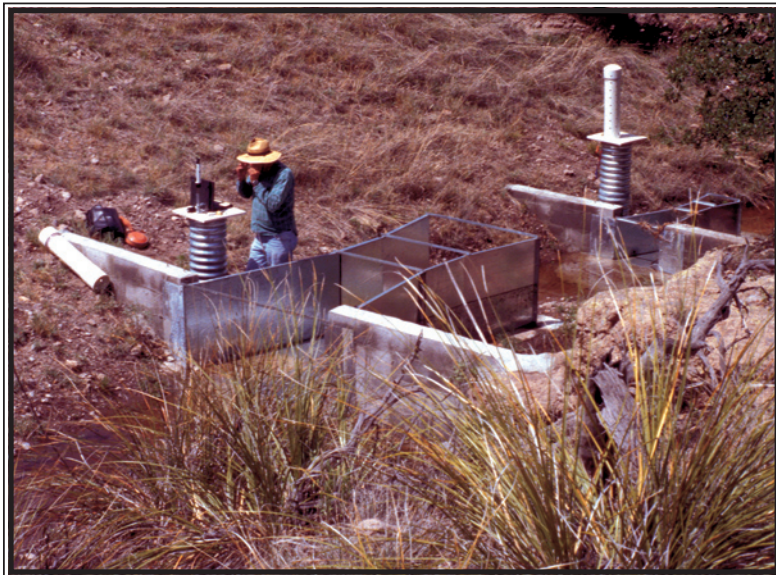
A forestry technician downloads hydrologic data to a laptop computer from a Parshall flume installation at the Cascabel Watersheds, New Mexico. The small flume measures typical low streamflow events and the larger flume measures higher events. The 12 small instrumented watersheds will be used to evaluate the effects of warm and cool season prescribed burning and unburned conditions on the physical, chemical, and biological components of the oak savanna ecosystem. (Photo by John Yazzie)
